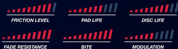
RST 1 has a very high friction level and high temperature resistance. Cold friction and initial bite makes this material most appropriate for Sprint Racing.
